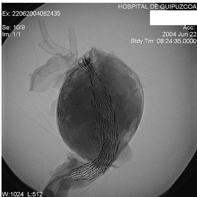
Fig. 4. Radiograph of collapsed thoracic aortic stent-graft and thoracic aorta explanted en bloc from deceased patient. Note multiple collapsed stents and migration of the stent-graft.
