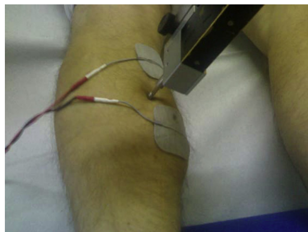
Figure 1. Electrodes and displacement sensor positioned for TMG measurements on the gastrocnemius medialis muscle.
